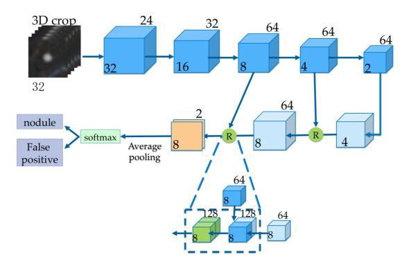
Fig.2 Structure of U-net Classifier Model
