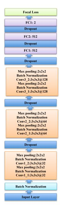
Fig.1 Structure of 3D-DCNN Model
