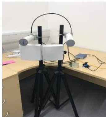
Fig. 1 – Typical radar configuration with transmitting and receiving antennas (the radar is the blue device on the table, and the two antennas are the white cylinders on the two support tripods)
